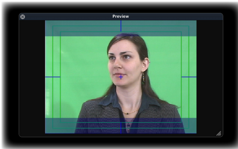
The Preview Palette with 16x9 mask, center marks, and title safe overlays enabled.
